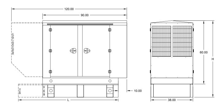
All enclosure models are 200 MPH wind rating certified in accordance with IBC2018 and ASCE/SEI 7-16 standards.
